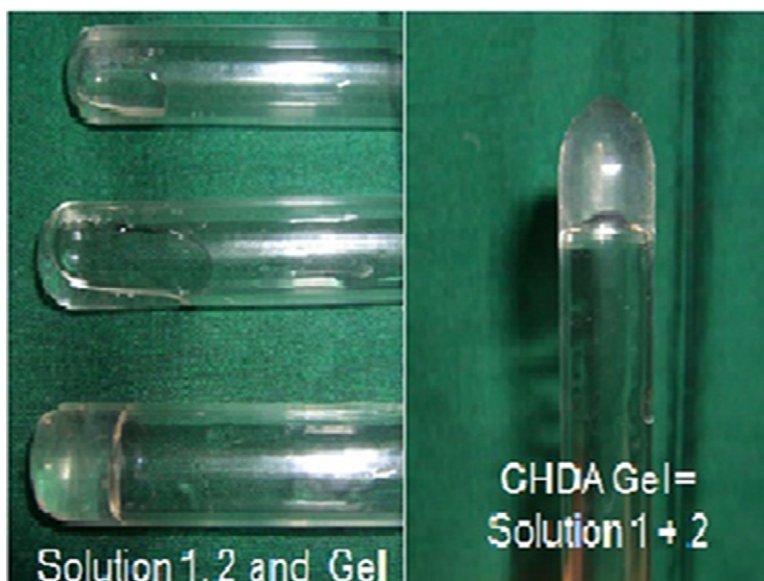
Fig. 1. Picture shows the gel formation when chitosan and HDA solutions are mixed in a test tube. Solutions 1 and 2 are chitosan and HDA solution, respectively.
